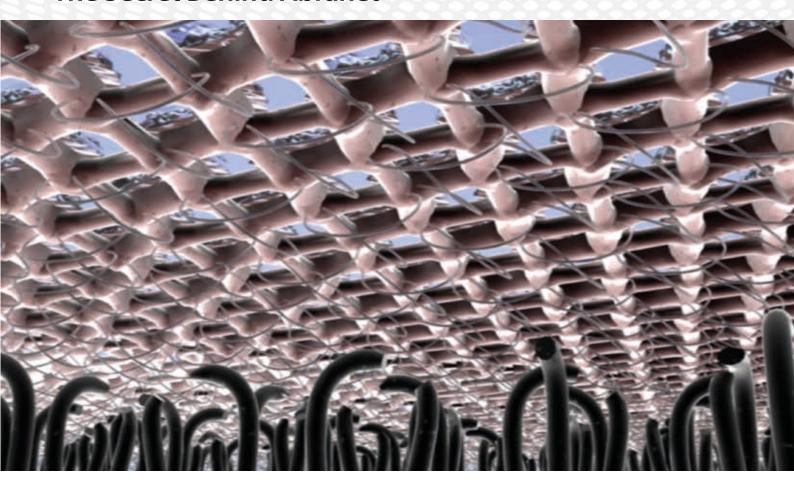
A modern production process requires a sanding material which is efficient and reliable. The open structure of Abranet prevents clogging and enables faster sanding. The patented construction consists of a dense network of polyamide fabric threads onto which the abrasive grit is bonded.
